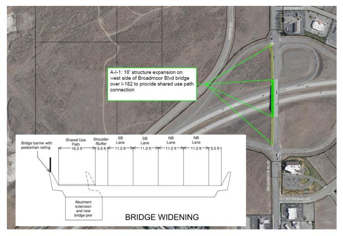
FIGURE 33: ALTERNATIVE A-I-1 (BROADMOOR BRIDGE WIDENING) CONCEPTUAL LAYOUT
