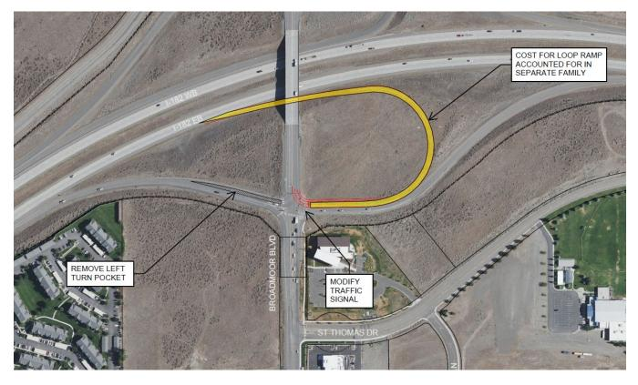
FIGURE 29: ALTERNATIVE E-S-1 (SIGNAL + LOOP RAMP) CONCEPTUAL LAYOUT
