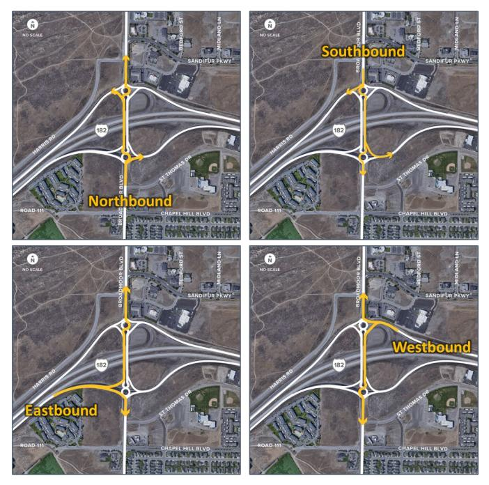
FIGURE 36: DDI WITH ROUNDABOUTS CIRCULATION DIAGRAM
