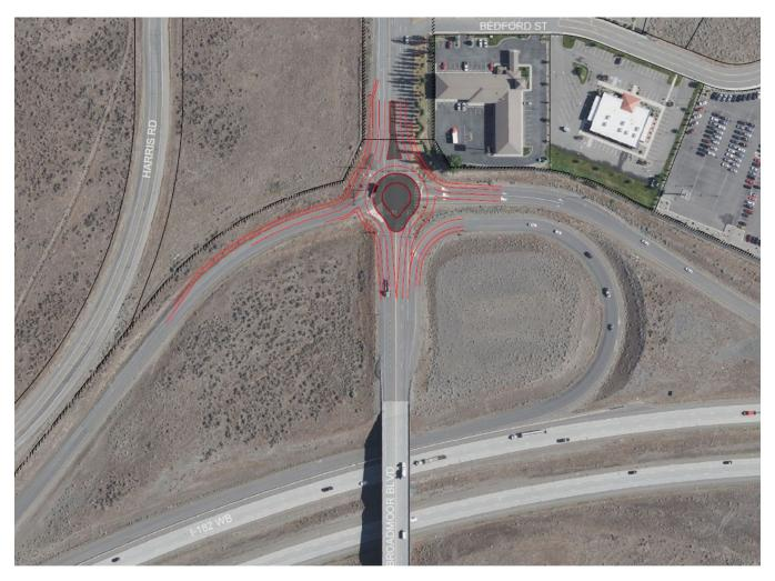
FIGURE 26: ALTERNATIVE W-R-1 (ROUNDABOUT) CONCEPTUAL LAYOUT
