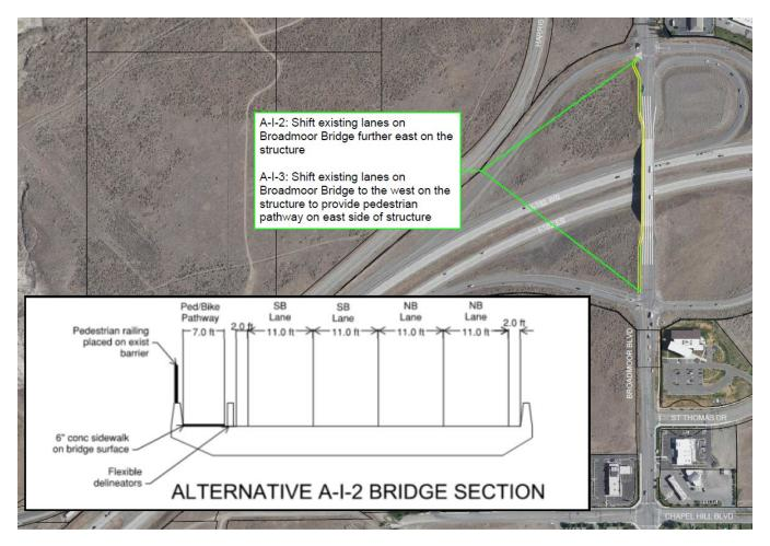
FIGURE 34: ALTERNATIVE A-I-2 (BROADMOOR RE-STRIPING) CONCEPTUAL LAYOUT
