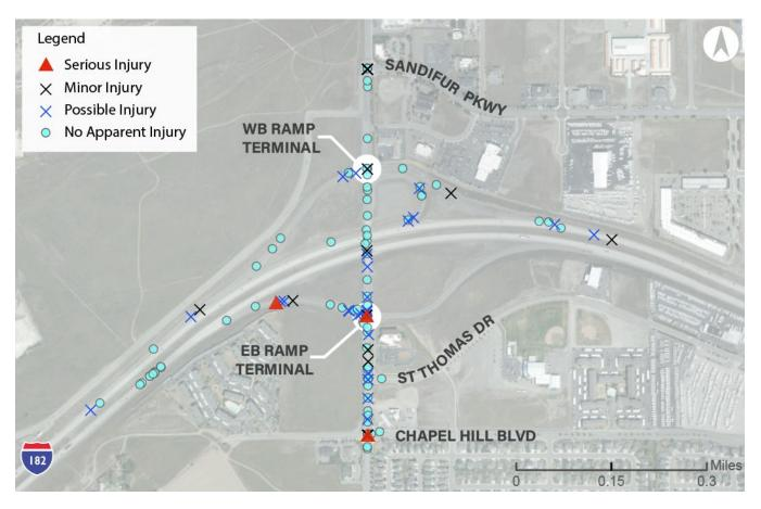
FIGURE 11: CRASH SEVERITY FOR ALL COLLISIONS ANALYZED ALONG STUDY CORRIDOR.
