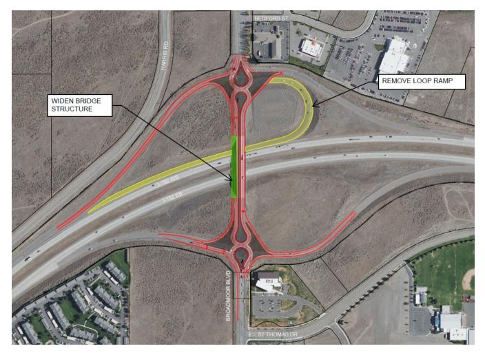
FIGURE 35: ALTERNATIVE C-P-3 (DDI WITH ROUNDABOUTS) CONCEPTUAL LAYOUT
