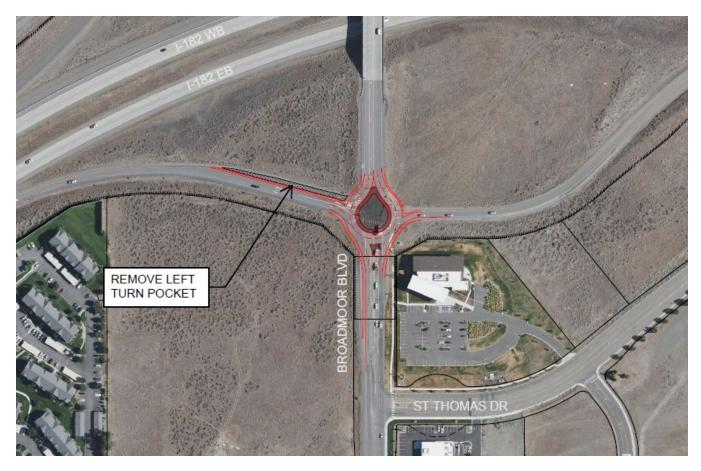
FIGURE 28: ALTERNATIVE E-R-2 (ROUNDABOUT) CONCEPTUAL LAYOUT
