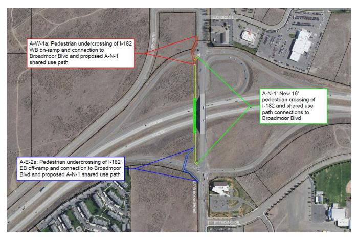
FIGURE 30: ALTERNATIVES A-N-1, A-W-1A, AND A-E-2A CONCEPTUAL LAYOUTS
