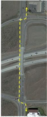
FIGURE 10: PROTECTED PEDESTRIAN ROUTE THRU INTERCHANGE
