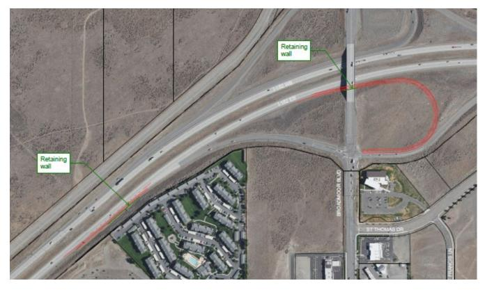
FIGURE 22: ALTERNATIVE F-E-2 (LOOP RAMP WITH DECEL. LANE) CONCEPTUAL LAYOUT
